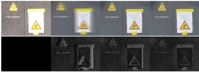
Figure 4. Two examples of laser scan renderings colored by differently aligned images. Top row, from left to right: Original laser scan colors, initial alignment, 7-DoF ICP alignment, our alignment. Bottom row: Difference of each image to the laser scan image. Note that the different lighting causes a significant color difference.
