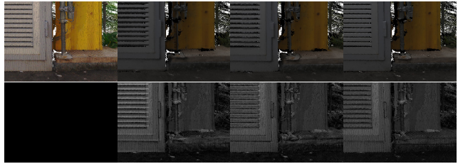
Figure 4. Two examples of laser scan renderings colored by differently aligned images. Top row, from left to right: Original laser scan colors, initial alignment, 7-DoF ICP alignment, our alignment. Bottom row: Difference of each image to the laser scan image. Note that the different lighting causes a significant color difference.
