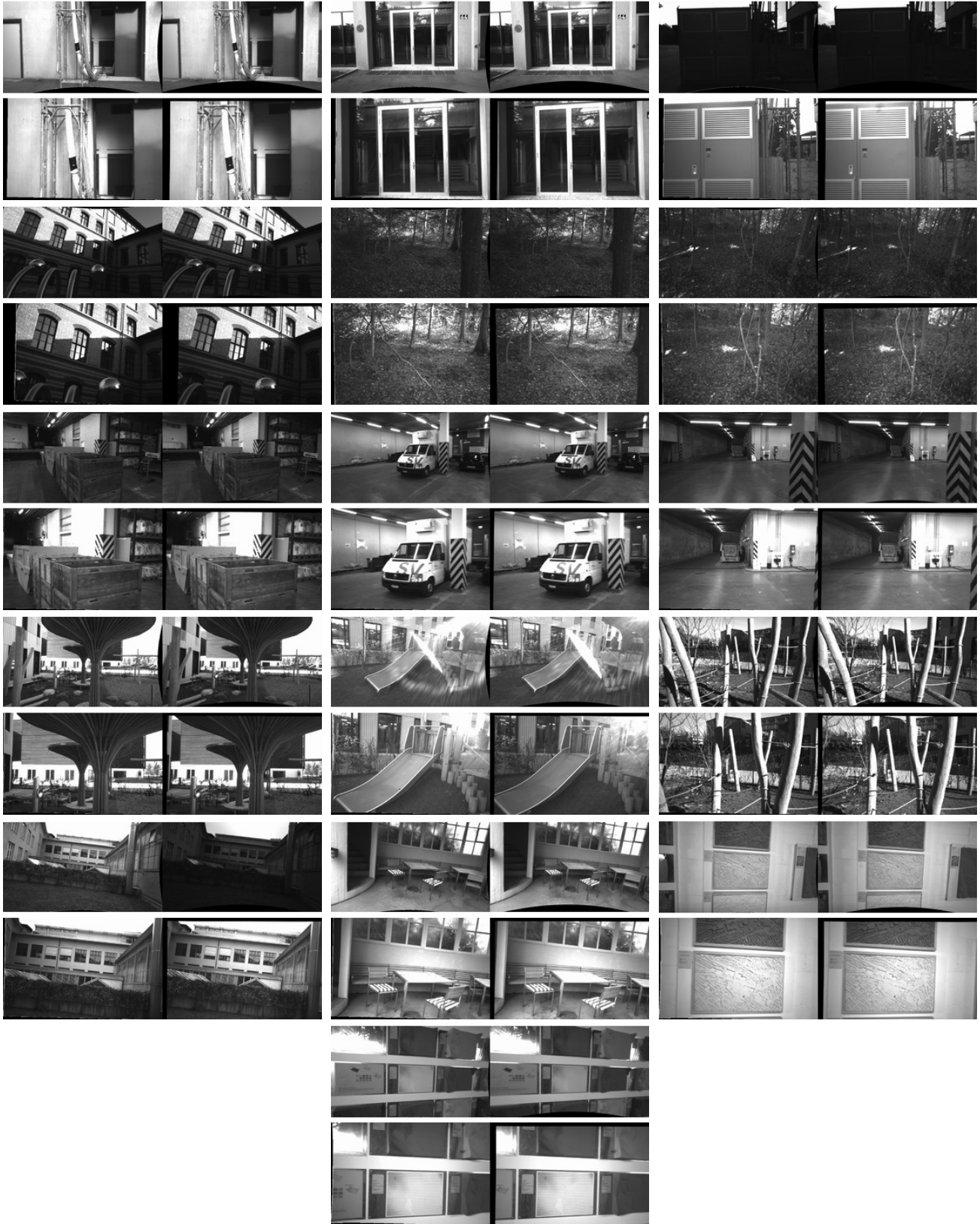
Figure 4: Low-resolution two-view stereo images, captured by two stereo pairs whose cameras have different fields-of-view. The images have been rectified.
